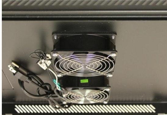
Cabinets Fans for Ventilation
