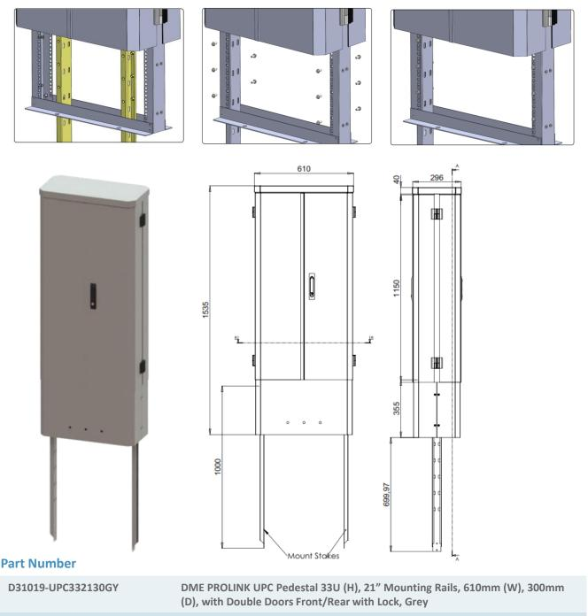
DME PROLINK Mounting Stake for UPC Pedestal, Grey / Dimension : 1000mm (L) X 57mm (W) X 25mm (D), 2mm (T) – 2 Nos. in one set
